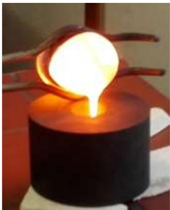
Pouring of molten glass in a graphite mould
