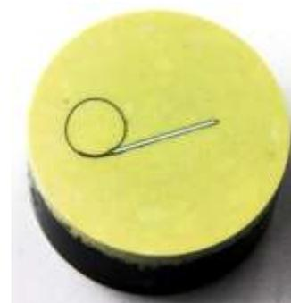
Metallographic detection layer on the alumina substrate-longitudinal section of the embedded pyrolytic graphite electrode with microsection
